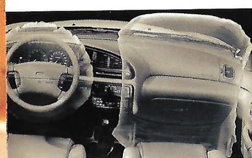
Standard Second Generation dual airbags are depowered to further enhance protection for the driver and passenger.
