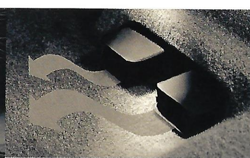
Flow-through heat ducts provide rear passenger comfort.
